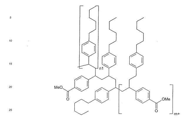
is low in aqueous solution, it is preferable to co-polymerize 4-ethenyl benzenesulfonate to increase the solubility of the precursor. The precursor is refluxed with a polyamine and the resulting methanol removed to produce the final polymer. The composition of the polymer may be varied to achieve desired properties.
