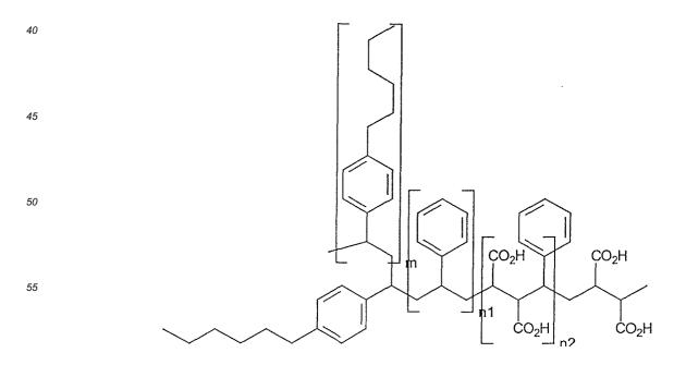
The hydrophobic block should have at least 6 mers, while the polyacid blocks should have at least 3, providing 6 acid functionalities. If a monofunctional carboxylate is used, the minimum number of mers should be increased. The molecular weight should be between 1,000 and 500,000.
