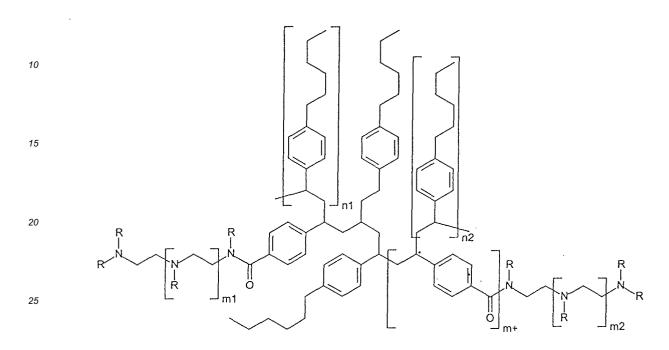
The poly(imine) groups facilitate adhesion of the ink through electrostatic interactions, while the phenylhexane side chains stabilize the dye/fixer complex against physical abrasion. Each block should have at least 6 mers, while m+ is a single mer linking the poly(imine) block to the poly(phenylhexane) block. The m+ mer also facilitates chain branching. The molecular weight should be between 1,000 and 500,000.
