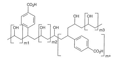
45 is combined with PEI via the benzoate groups to form the polymer of Example 3, or with some other polyamine, through a condensation reaction.
