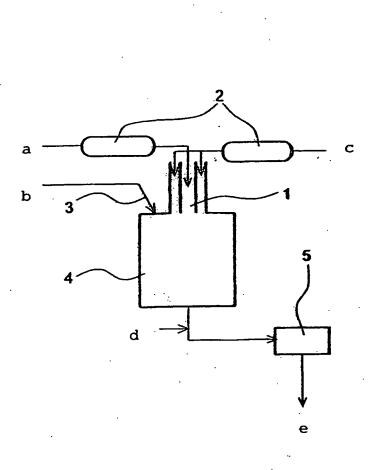
a...TITANIUM TETRACHLORIDE (AND DILUTING GAS) b...AQUEOUS SALT SOLUTION CONTAINING METAL ELEMENT c...OXYGEN AND WATER VAPOR
