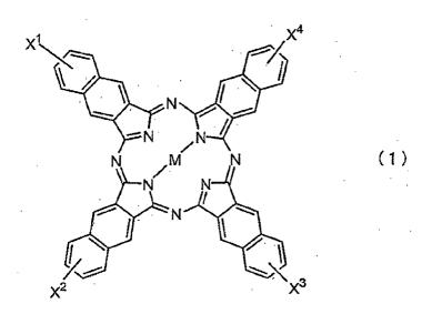
where, in the formula (1), M represents two hydrogen atoms, or a metal atom, provided that the metal atom may have a ligand, and each of X<sup>1</sup>, X<sup>2</sup>, X<sup>3</sup> and X<sup>4</sup> is a hydrogen atom or a substituent.
