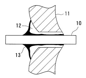
Section at tube/header joint (after 480 hours of CASS test)
