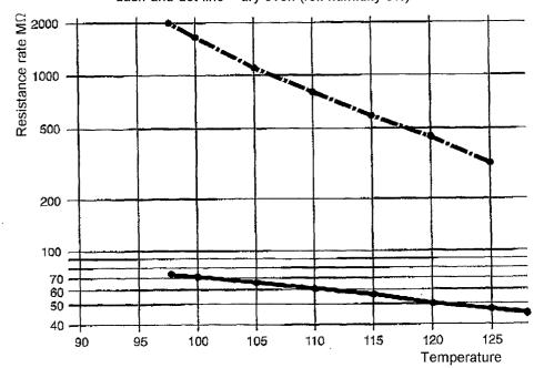
**[0011]** Since the meter has been modified by an external voltage source, the measuring results are not truthful, yet provide an idea regarding the transition of impedance according to temperature and humidity.
