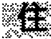
IMAGE OBTAINED BY ELIMINATING A HALF-TONE DOT, THE SIZE OF WHICH IS SMALLER THAN A SPECIFIC VALUE ACCORDING TO THE PRIOR ART (b)
