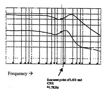
Resonant point of inductor 116 and blocking capacitor  $100 \cong 1.7 \text{KHz}$
