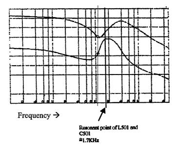
Resonant point of inductor 116 and blocking capacitor  $100 \cong 1.7 \text{KHz}$
