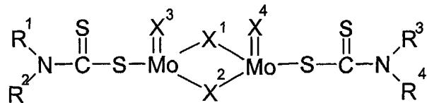
10 wherein R<sup>1</sup>, R<sup>2</sup>, R<sup>3</sup> and R<sup>4</sup>, are independently selected from a hydrocarbon group; X<sup>1</sup> to X<sup>4</sup> are independently selected from sulfur or oxygen atom; wherein said molybdenum dithiocarbamate is present below 175 ppm in terms of molybdenum concentration, based upon the total mass of the composition.
