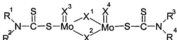
40 wherein R<sup>1</sup>, R<sup>2</sup>, R<sup>3</sup> and R<sup>4</sup>, are independently selected from a hydrocarbon group; X<sup>1</sup> to X<sup>4</sup> are independently selected from sulfur or oxygen atom; wherein said molybdenum dithiocarbamate is present below 125 ppm in terms of molybdenum concentration, based upon the total mass of the composition;
