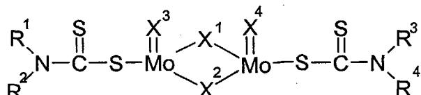
20 wherein R<sup>1</sup>, R<sup>2</sup>, R<sup>3</sup> and R<sup>4</sup>, are independently selected from a hydrocarbon group; X<sup>1</sup> to X<sup>4</sup> are independently selected from sulfur or oxygen atom; wherein said molybdenum dithiocarbamate is present below 175 ppm in terms of molybdenum concentration, based upon the total mass of the composition.
