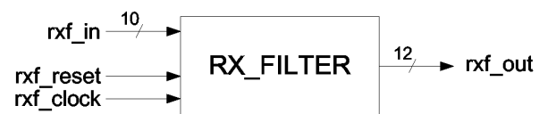
Figure 72: downlink reception: shaping filter
