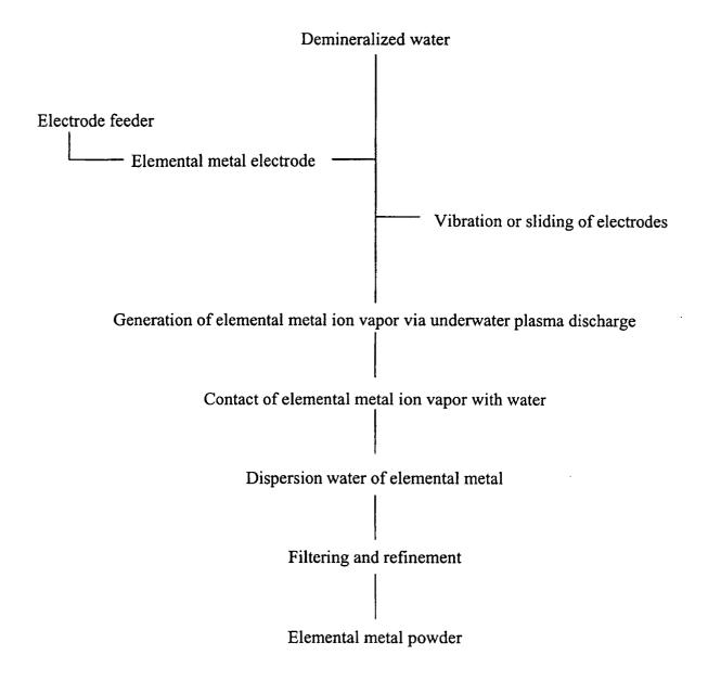
Apparatus for Producing Metal Powder Proposed by the Present Invention
