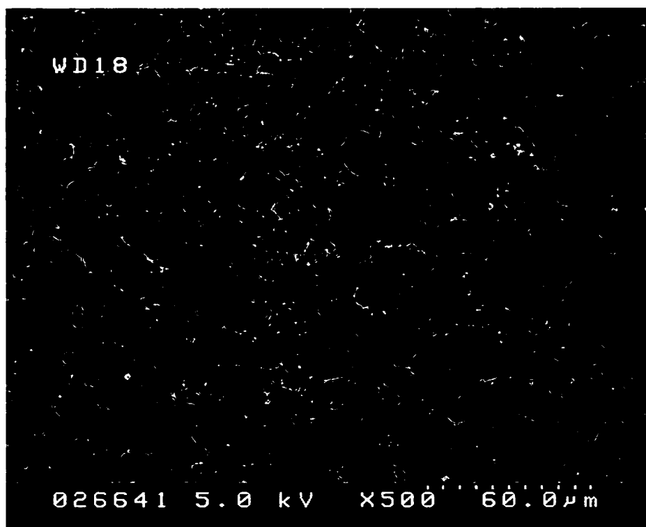
SEM PHOTOGRAPH SHOWING SURFACE OF BINCHOTAN CHARCOAL
