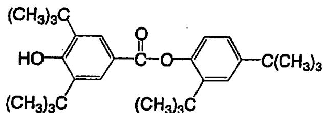
35 [0111] In view of effectively improving an image retention property, a content of the ultraviolet light absorber in a single thermosensitive recording layer is preferably 10-300 parts by mass, more preferably 30-200 parts by mass relative to 100 parts by mass of the electron-donating colorless dye.
