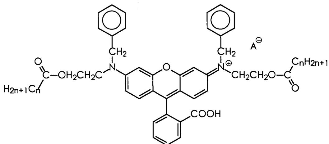
40 wherein A is the anion corresponding to the acid used for protonation. The zwitterionic form of this colorant is believed to be of the formula
