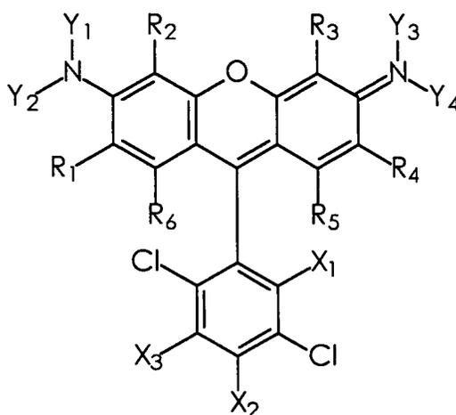
wherein R<sub>1</sub>-R<sub>6</sub> are hydrogen, fluorine, chlorine, lower alkyl lower alkene, lower alkyne, sulfonate, sulfone, amino, amido, nitrile, lower alkoxy, lining group, or combinations thereof or, when taken together, R<sub>1</sub> and R<sub>6</sub> is benzo, or, when taken together, R<sub>4</sub> and R<sub>5</sub> is benzo; Y<sub>1</sub>-Y<sub>4</sub> are hydrogen or lower alkyl or, when taken together, Y<sub>1</sub> and Y<sub>2</sub> is propano and Y<sub>2</sub>
