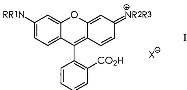
wherein  $R_1$ ,  $R_3$  are each lower alkyl;  $R_2$  is lower alkyl, 10C or higher long-chain alkyl;  $R_4$  is 10C or higher long-chain alkyl;  $X^-$  is an anion, or squarylium compounds of formula II
