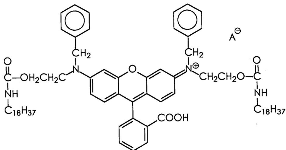
wherein A is the anion corresponding to the acid used for protonation. The zwitterionic form of this colorant is believed to be of the formula
