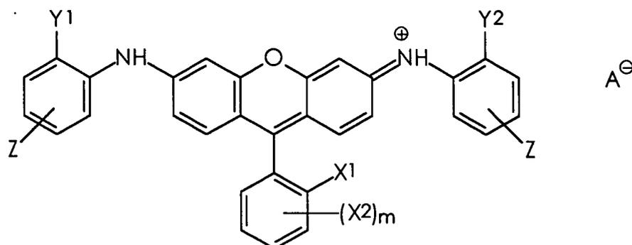
wherein  $X^1$  is an ester group or an amide group (such as of a carboxylic or sulfonic acid) or a fatty amine salt of a sulfonic acid, each  $X^2$  independently is a substituent,  $m$  has a value of from 0 to 2,  $Y^1$  and  $Y^2$  are each independently H, alkyl, or halo, each  $Z$  independently is an ester or amide group, and  $A^-$  is an anion. The compound is useful as a colorant for toners, D2T2 printing, plastics, polyesters, nylons, and inks, especially ink jet or hot melt inks.
