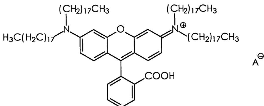
wherein A is the anion corresponding to the acid used for protonation. The zwitterionic form of this colorant is believed to be of the formula
