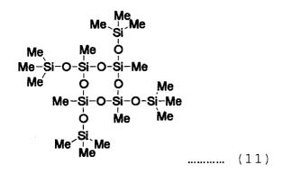
**[0059]** The results of NMR analysis of the monomer (A-7) thus obtained are as follows:  $^{1}\text{H-NMR}(300\text{MHz}, \text{ in acetone-d}_{6}): \delta 0.059(\text{s}, 36\text{H}, 4\times[\text{-CH}_{3}]_{3}), 0.092(\text{s}, 12\text{H}, 4\times[\text{-CH}_{3}]).$
