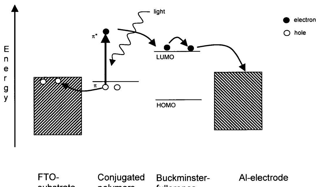
Fig. 1: Schematic band diagram and different excitation processes of and in solar cells based on Buckminsterfullerenes.
