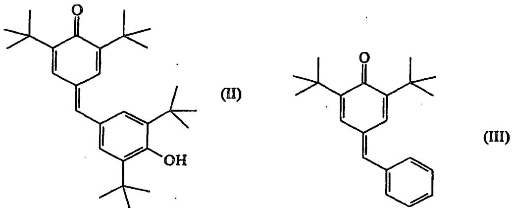
15 [0017] In the present invention, a single quinone methide may be used, or it may be used in combination with different quinone methides. The quinone methide composition may be added at or upstream of any point where viscosity increase 30 or fouling may occur. This includes either to the oil quench tower, specifically to the upper section and bottom section of the oil quench tower, or at any point upstream of the oil quench tower. The composition is added during the ethylene production.
