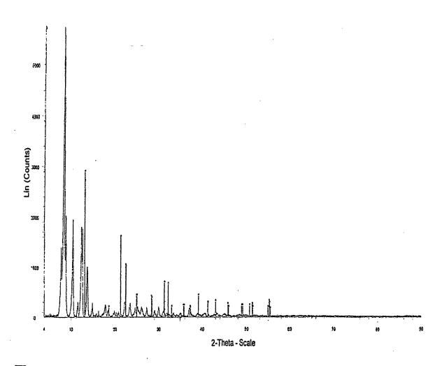
Centre of x-ray diffraction spectrum-File: CB47.raw - Type 2ThTh locked - Start:4.000' - End: 90.000' - Step: 0.020' - Step time: 2.4s - Temp: 27°C - Time started: 30s - 2-Theta: 4.000' - Theta: 2.000' - Chi: Operations Backround 1.000, 1.000 Import
