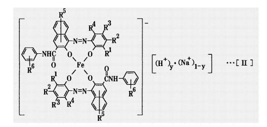
(in the chemical formula [II],  $R^1$ -,  $R^2$ -,  $R^3$ -,  $R^4$ -,  $R^5$ - and  $R^6$ - are the same above; y is mole ratio and 0 to 0.2); a step for filtrating, washing and drying the azo-type iron complex salt, said iron-complexing step with the monoazo compound is carried out in mixed solvent of a lower alcohol having 1 to 6 carbon atoms and water included at least 70% by weight thereof.
