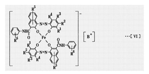
(in the chemical formula [VI], B<sup>+</sup> is  $(H^+)_X(Na^+)_{1-X}$  and x is mole ratio and 0.6 to 0.9, or B<sup>+</sup> is  $(H^+)_Y(Na^+)_{1-Y}$  and y is mole ratio and 0 to 0.2) and the aggregate particles have 0.5 to 5.0 microns of an average particle size. A toner for developing an electrostatic image comprises a resin for the toner and the charge control agent. An image formation process of
