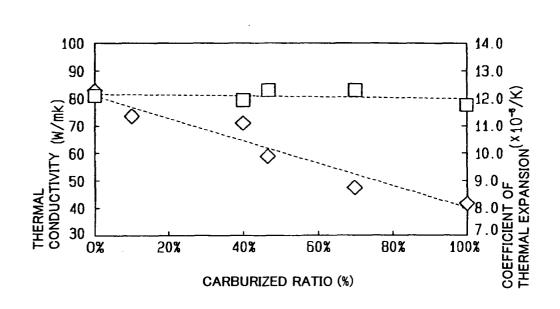
♦: THERMAL CONDUCTIVITY RELATIVE TO CARBURIZED RATIO
