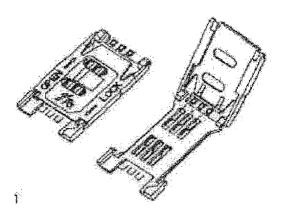
Figure 1: Connectors(Closed/Open) for the control card
