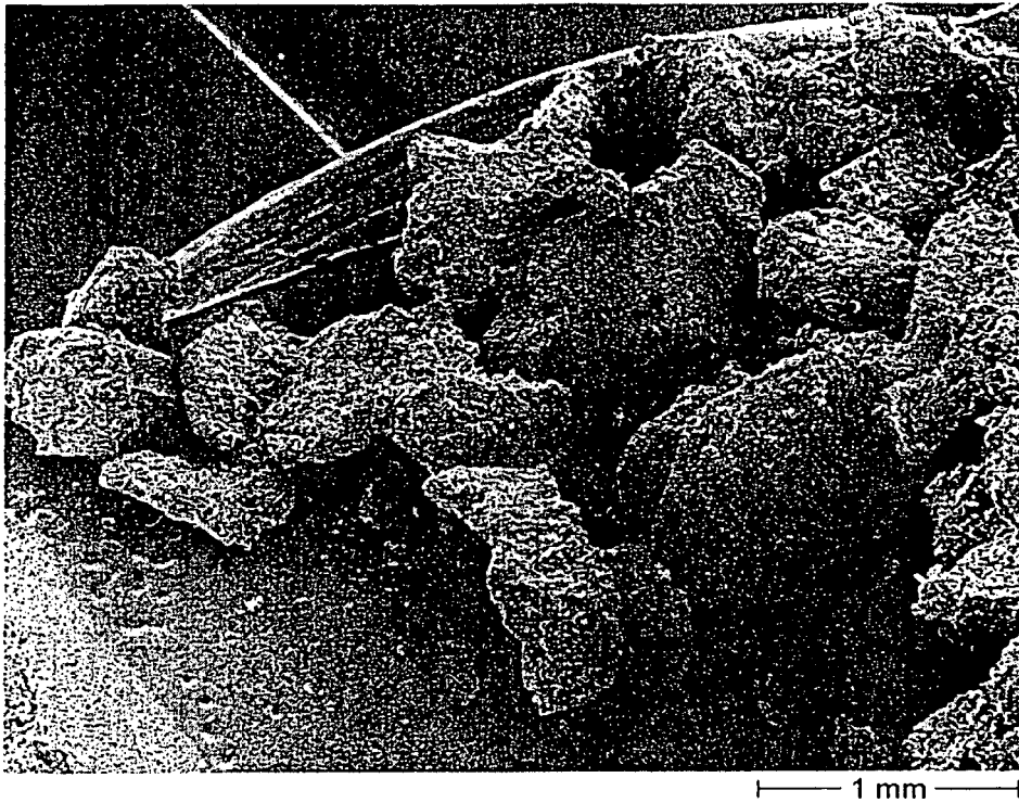
Figure 13B: Surface of Nal-Extr granulates at 200x magnification. The voltage was 10 kV. The bar length corresponds to 100 \mu m.
