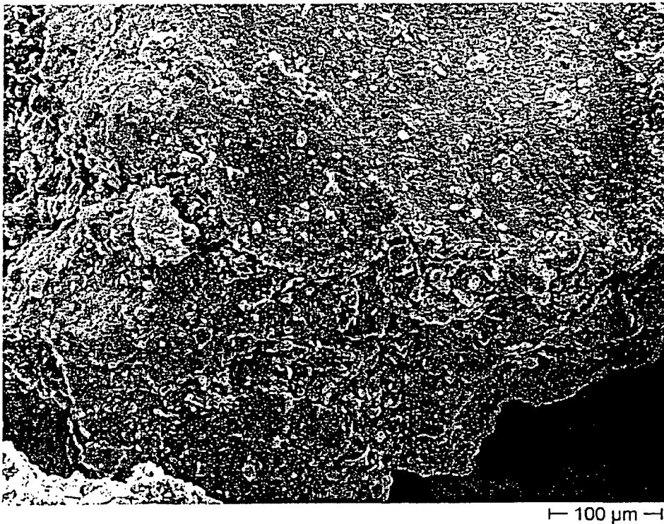
Figure 13B: Surface of Nal-Extr granulates at 200x magnification. The voltage was 10 kV. The bar length corresponds to 100 \mu m.
