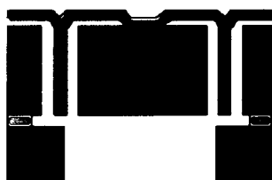
8. Release in vapor phase HF
