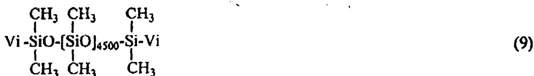
55 and 95 parts of the dimethylpolysiloxane with both terminals blocked with dimethylvinylsiloxy groups and with a viscosity of 1,000 mPa·s (H/Vi was 0.5), preparation and curing in the same manner as the comparative example 1 yielded a cured product with a penetration value of 60.
