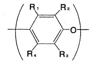
wherein O denotes an oxygen atom, and  $R_1$  to  $R_4$  each independently denote hydrogen, halogen, primary or secondary lower alkyl, phenyl, haloalkyl, aminoalkyl, hydrocarbonoxy, or halohydrocarbonoxy, with a proviso that at least two carbon atoms are between a halogen atom and an oxygen atom.
