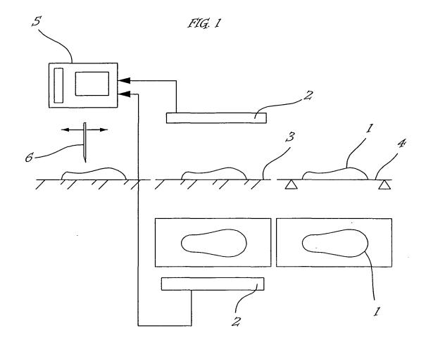
**[0001]** The present invention relates to a process for forming cheese parts having fixed weight, particularly to irregular shaped cheeses which are difficult to be cut by automatic devices adapted to produce pieces having the same weight.
