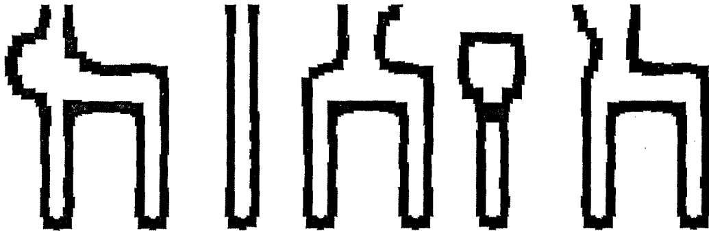
Figure 17. Single-layer pv-Band interaction. The internal and external distances of the pv-Bands determine the pass-fail criterion.
