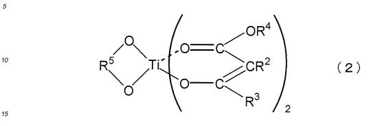
20 wherein R<sup>2</sup>, R<sup>3</sup> and R<sup>4</sup> are the same as defined above, R<sup>5</sup> is a substituted or unsubstituted divalent hydrocarbon group having 1 to 20 carbon atoms.
