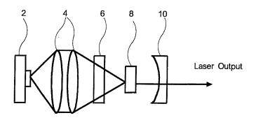
2: 1W LaserDiode 4: Lense 6: HR 8: Nd:Lu2O3 10: OC:T-3% (808nm) f=8mm Ceramics R=50mm
