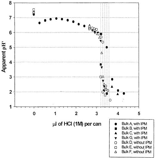
Effect of hydrochloric Acid on Acidity Function (pH') of Formoterol Fumarate Solution ( $12\mu g/100\mu l$ ) in Vertrel XF/HFA containing 12% w/w Ethanol
