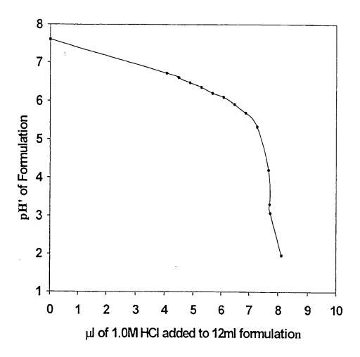
Effect of hydrochloric acid on Acidity Function (pH')of Formoterol Furnarate Solution ( $12\mu g/100\mu l$ ) in Vertrel XF/HFA containing 20% w/w Ethanol.
