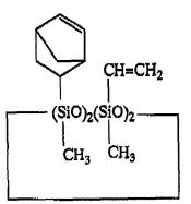
**4.** The composition according to any one of claims 1, to 3, wherein the polycyclopolysiloxane (B) has the following repeating units.
