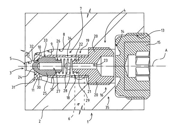
[0001] The present invention relates to a high-pressure fuel pump for an internal combustion diesel engine. [0002] In particular, the present invention relates to a high-pressure fuel piston pump for feeding fuel to a common rail of an internal combustion diesel engine.
