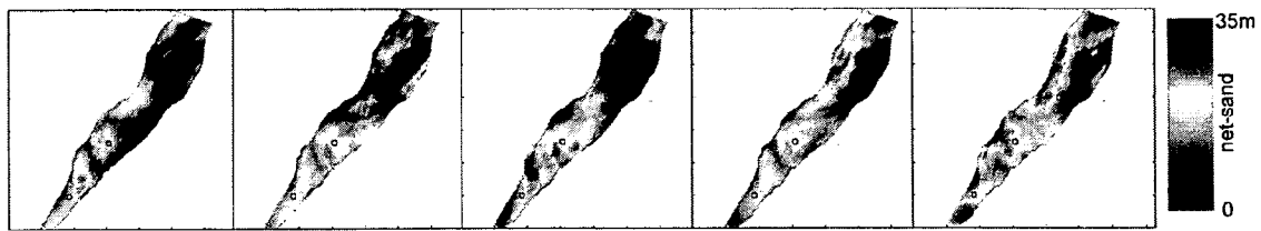
(a) 5 realisations of net-sand in plan view
