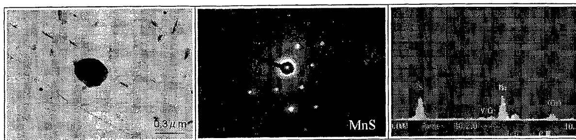
Fig. 2 A sulfide observed in the ASME P92 steel
