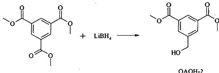
25.2 g (0.1 mol) of trimethyl 1,3,5 benzenetricarboxylate was dissolved in 85 mL of methyl acetate at 50°C. 40.5 ml (0.08 mol) lithiumborohydride 2.0 M in THF was added drop wise and the mixture was stirred during 3 hour at 50°C. After this period 5.3 gram acetic acid (0.088 mol) and 3 mL water were added. The methyl acetate and THF were evaporated, 50 ml water and 50 ml n-hexane were added. The product QAOH-2 was filtered and washed with a small volume water and n-hexane. The yield was 63%.
