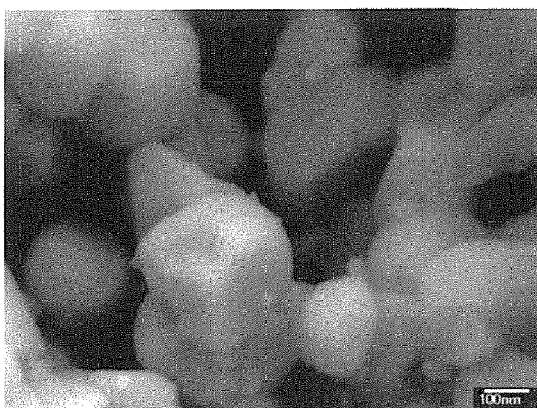
FIG. 4: Evolution of a 5 wt.% Rh catalytic material nanostructure as a function of the thermal treatment in the frame of the process described in Figure 3a
