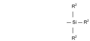
where R<sup>2</sup> is an alkoxy of 2 to 4 carbon atoms, alternatively 2 carbon atoms; alk is a divalent hydrocarbon of 2 to 4 carbon atoms, alternatively with 3 carbon atoms; and n is an integer of from 2 to 5, alternatively 2 or 4.
