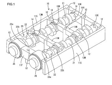
[0001] This invention relates to a supporting structure and a supporting member for a camshaft.
