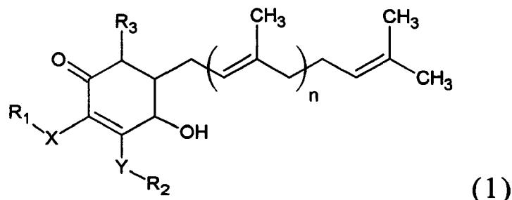
15 wherein X and Y can be oxygen or sulfur, R<sub>1</sub>, R<sub>2</sub> and R<sub>3</sub> are each a hydrogen atom, methyl or (CH<sub>2</sub>)<sub>m</sub>-CH<sub>3</sub> and m=1-12; n=1-12.
