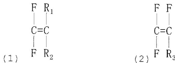
In the formula (1), R<sub>1</sub> and R<sub>2</sub> each independently represent a hydrogen atom or fluorine atom. In the formula (2), R<sub>3</sub> represents a substituent represented by C<sub>n</sub>H<sub>2n+1</sub> (in which n is an integer of 1 or more).
