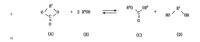
wherein R<sup>1</sup> represents a bivalent group -(CH<sub>2</sub>)<sub>m</sub>- (m is an integer from 2 to 6), one or more of the hydrogens thereof being optionally substituted with an alkyl group or aryl group having 1 to 10 carbon atoms. Moreover, R<sup>2</sup> represents a monovalent aliphatic group having 1 to 12 carbon atoms, one or more of the hydrogens thereof being optionally substituted with an alkyl group or aryl group having 1 to 10 carbon atoms.
