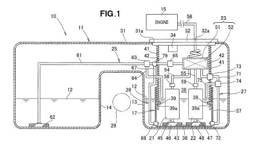
**[0001]** The present invention relates to a vehicle fuel supply device for supplying an engine with fuel that is stored in a main chamber and an auxiliary chamber of a saddle-shaped fuel tank.
