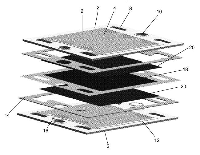
[0001] The present invention relates to a bipolar plate for polymer membrane (PEM) fuel cells.
