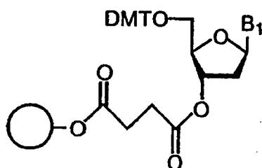
[0027] Herein, in the above-described structural formula, the circle represents the porous resin particle containing an aromatic vinyl compound-aromatic divinyl compound copolymer having a hydroxyl group, which is obtained by the method of the present invention, DMTO represents a protective dimethoxytrityl group at the 5'-position, and B<sub>1</sub> represents a base.
