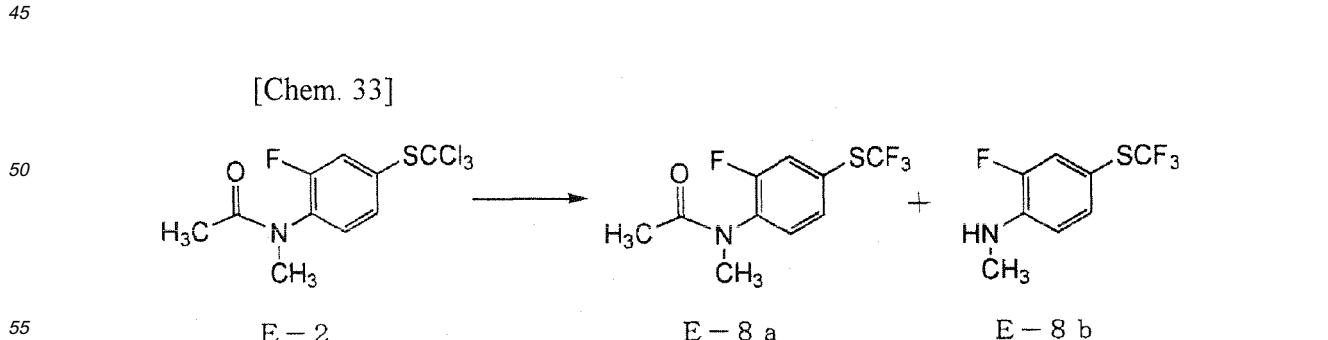
[0118] An autoclave was charged with a mixture of 0.32 g of N-acetyl-N-methyl-2-fluoro-4-trichloromethylthioaniline
