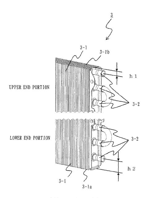
h1: DISTANCE BETWEEN UPPER END FACE OF FINS 3-1b AND CENTER OF UPPERMOST HEAT TRANSFER TUBE 3-2
