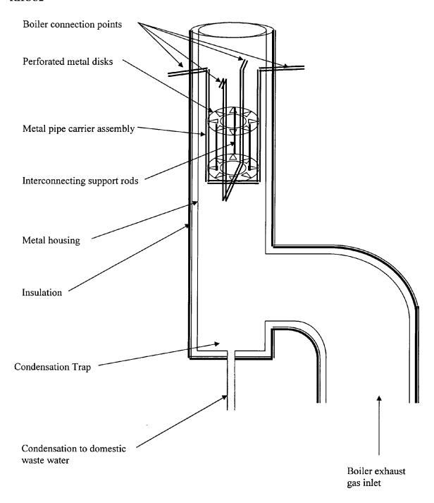
RHCU2 - Connected to Boiler - Not to scale
