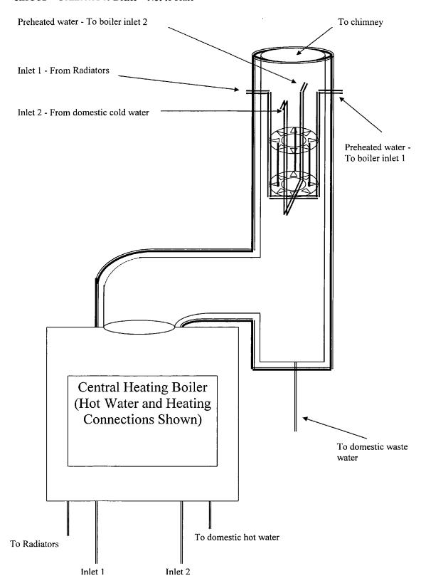
For single function boilers the RHCU2 inlets and outlets will be bridged together
