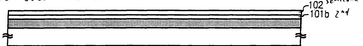
Fig.1D CRYSTALLIZATION OF SEMICONDUCTOR FILM 102
