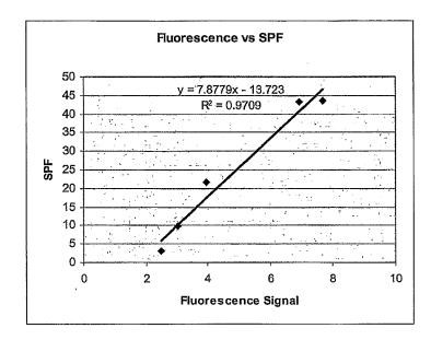
**[0085]** In this example, a threshold fluorescent level of at least 6 would be required to indicate that sufficient sunscreen had been applied to the skin. The diagnostic tool would then indicate a "Yes" signal, that sufficient sunscreen was in place. The indicator may be a green glowing light, or a LCD indicator, or a "meter" showing "Good". Fluorescence below
