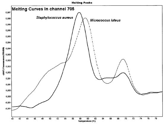
Melting curve analysis in channel 705 for Staphylococcus aureus (solid line; positive amplification signal in channel 640, negative in channels 610 and 670) and Micrococcus luteus (dotted line; positive amplification signal in channel 670, negative in channels 610 and 640).
