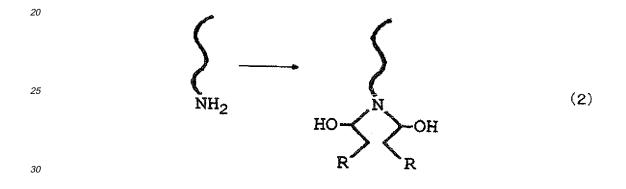
**[0030]** Since a part of or all of the terminal amino groups of the polyamide resin (A) changes to another group as a result of the reaction, the extrusion load during the extrusion molding into a film can be reduced while maintaining the fluidity, even if a large amount of the modified rubber (D) having an acid anhydride group or epoxy group is added.
